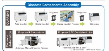
Convert manual insertion process to SMT inline process Reduce processes / dip solder investment
